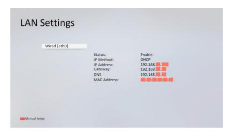
If there is a 0, press the red button (Manual Setup), choose the DCHP option and press OK (Save).
